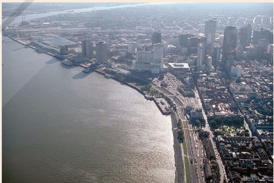
▶ FIGURE 12-21. New Orleans, the major shipping center on the lower Mississippi River, is protected by levees so that the river now stands 4 meters above the downtown area.
