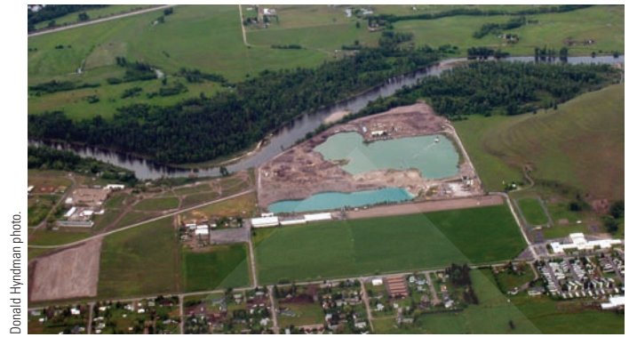
► FIGURE 12-36. Now flooded, these gravel pits along the South Platte River near Denver, Colorado, are only separated from the river by thin gravel barriers.
