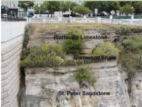
► Figure UMV-WSB.32 Exposure of the St. Peter Sandstone, Glenwood Shale, and Platteville Limestone at the Wabasha Street bridge, north bank of the Mississippi River, in downtown St. Paul, Minnesota.
