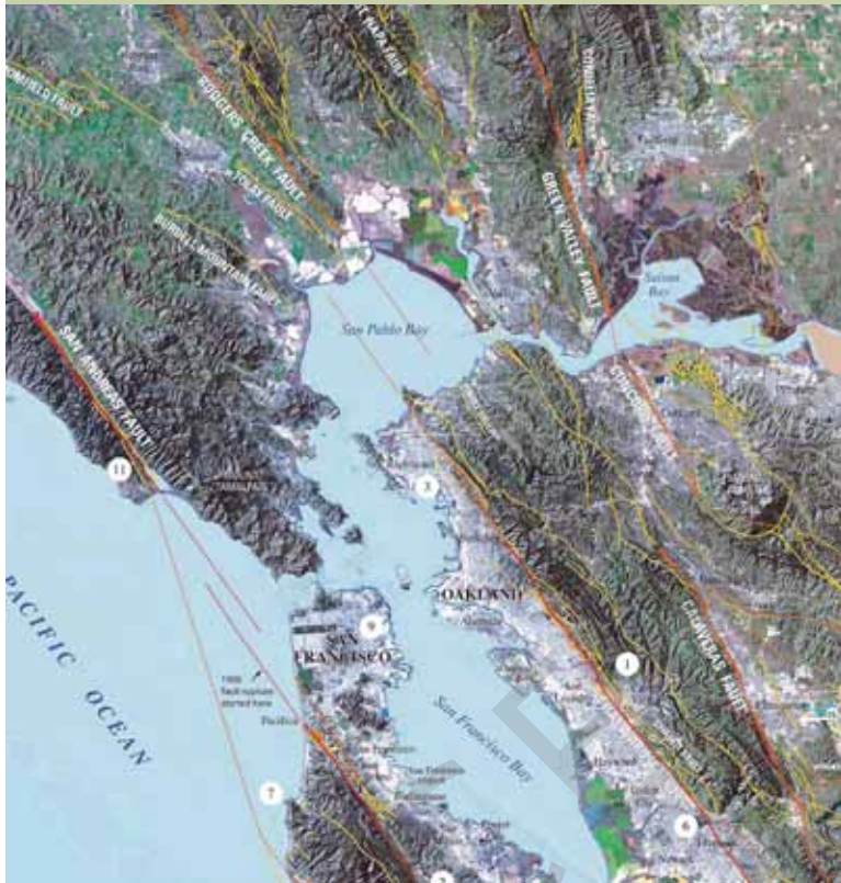
► Figure NC.54 Major faults of the San Andreas system in the San Francisco Bay Area. This map from the United States Geological Survey also identifies features resulting from recent offset along these faults by the circled numbers.
