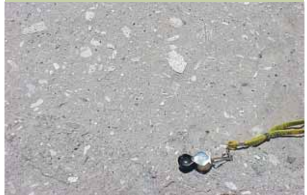
► Figure NC.13 Oligocene tuff near Soda Springs, California consists of ash particles and white pumice fragments welded into a coherent rock.
