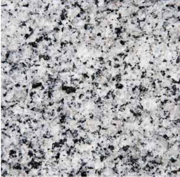
► Figure NC.6 Close up of granite from the Sierra Nevada Batholith. Dark crystals are biotite and hornblende, white crystals are plagioclase and potassium feldspar, and the gray translucent crystals are quartz.
