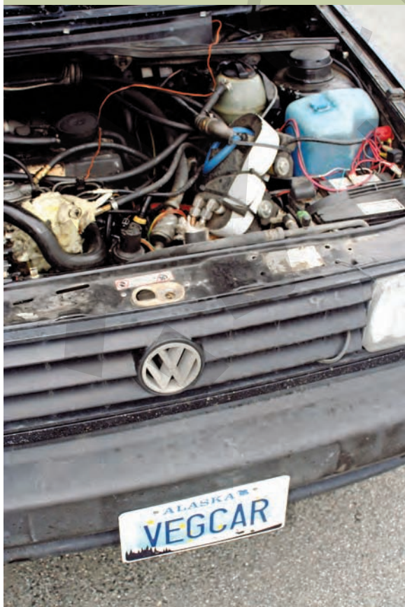
► Figure Carbon Cycle and Climate Change.23 The “VEGCAR,” a car whose engine has been modified to run on used vegetable oil (a biofuel).
