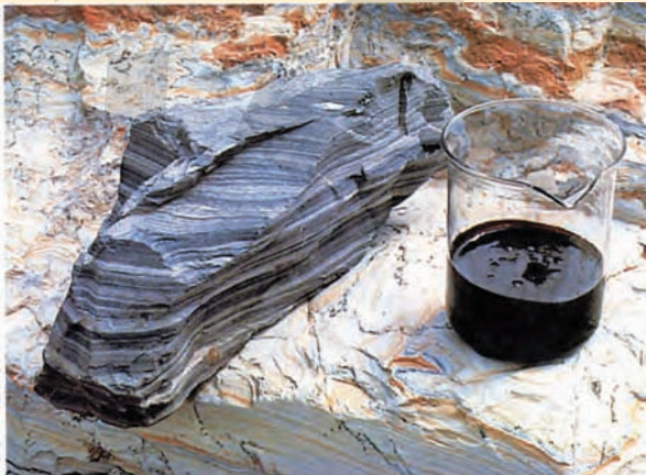
c Crude oil extracted from hydrocarbon-rich shale.
